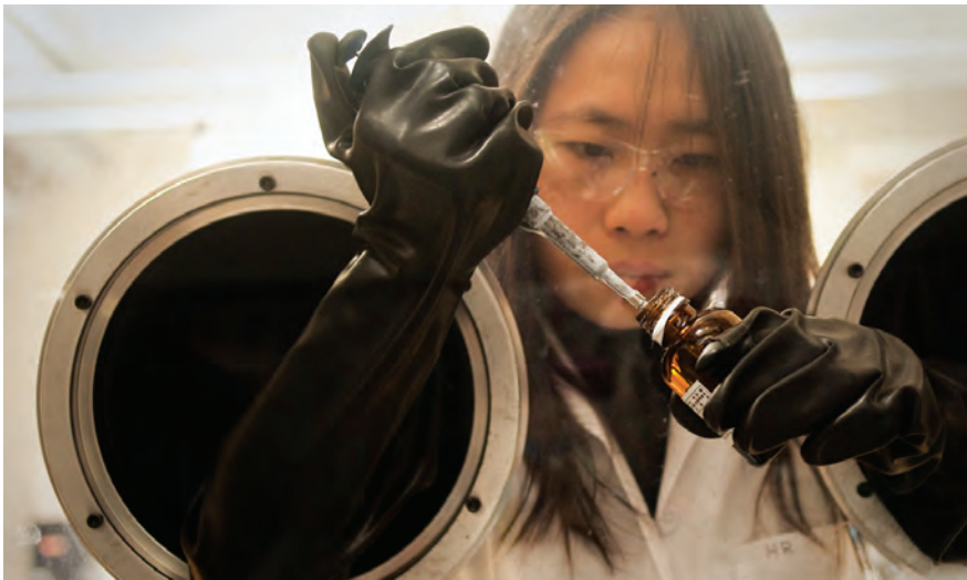
Doctoral student Yi-Chun Lu preparing electrolyte for lithium air battery testing
