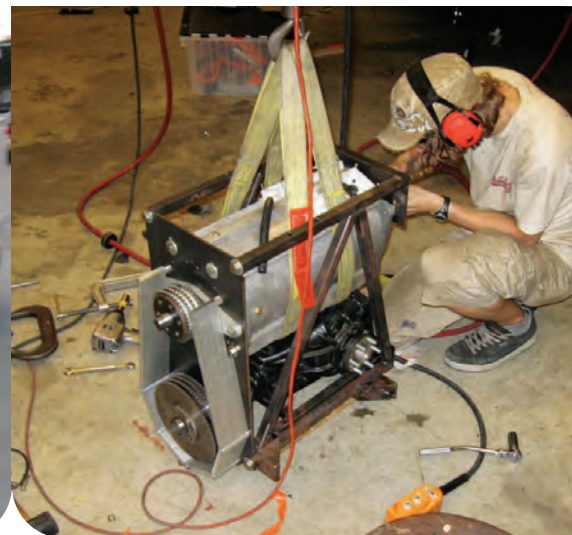
Mechanical Engineering sophomore Mike Nawrot trimming the alignment of the 250-horsepower drivetrain
