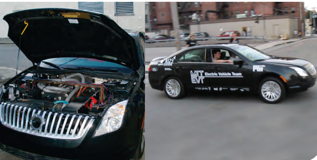
Under the hood after conversion to battery power
