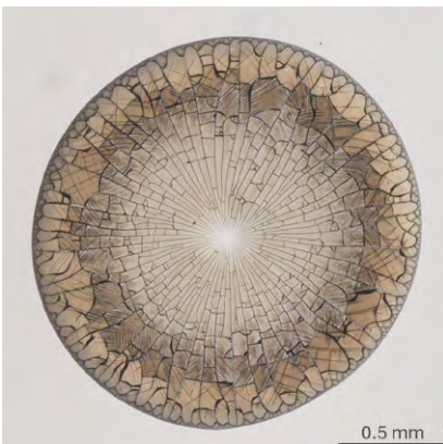
Crack patterns formed by drying drops of a colloidal suspension from Bischofberger's research. Credit: The researchers
