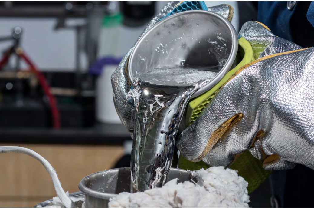
Molten tin stores heat and can be used to generate on-demand electricity. Credit: Rob Felt, Georgia Tech
